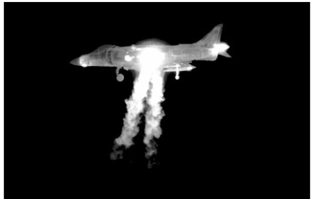
Images of a helicopter and Harrier jet taken with the ISCO403-based InSb SC6700 FLIR camera.
