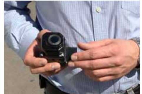
The FLIR PathFindIR is very compact and the rugged design keeps the vital core well protected against humidity and water, an important reason for Rosenbauer to choose this thermal imaging camera.
