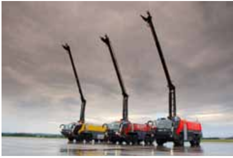
The Stinger's hydraulic arm has a reach of 16.5 meters high.
