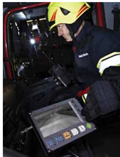
The thermal images from the FLIR PathFindIR are shown on the multifunctional screen in the cabin of the vehicle.
