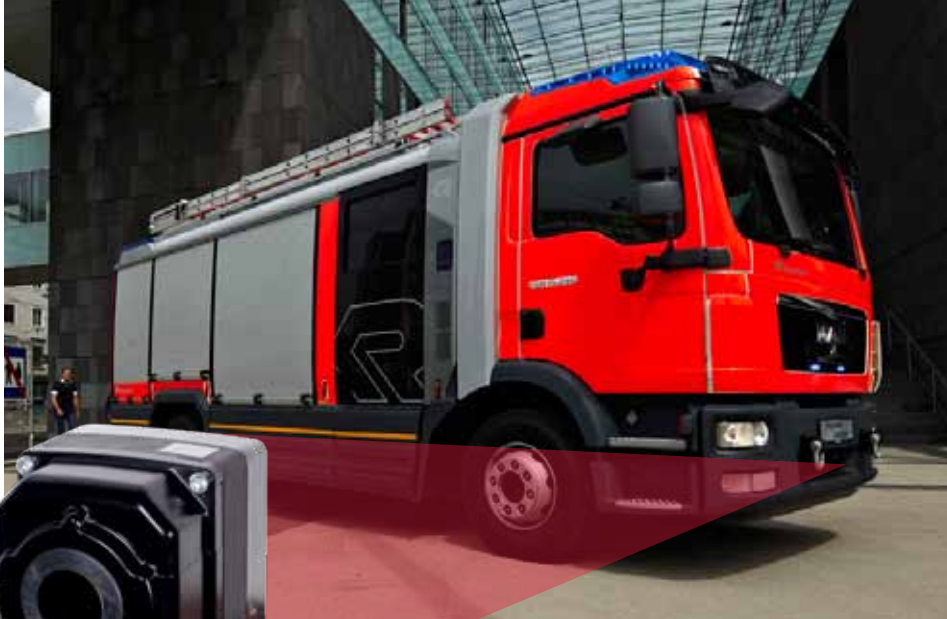
This new fire engine from the Rosenbauer's AT-Series has a FLIR PathFindIR thermal imaging camera installed in the bumper to help the firefighters see through smoke, which is especially useful in case of tunnel-fires.
